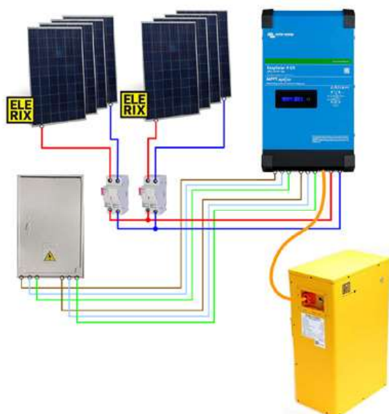
Single-phase hybrid PV plant
